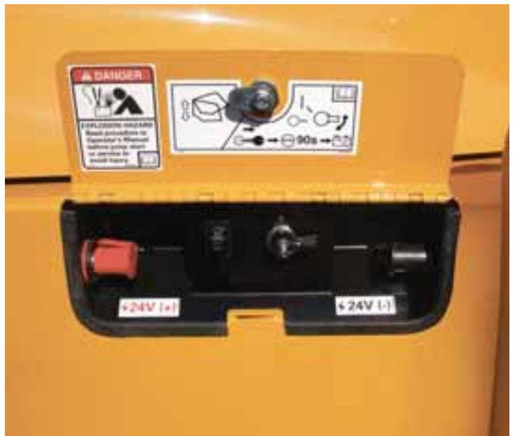
Hood opening and battery on/off switches. In case of flat battery, hood opening can be done externally with remote jump start
